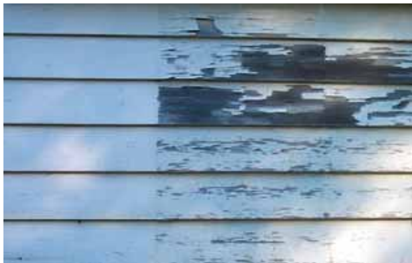
This picture shows a wooden panel that has been several years on the testing field. The section on the left was treated immediately, the one in the middle after 6 months and the one on the right 1 year after the panel was installed on the testing field.
